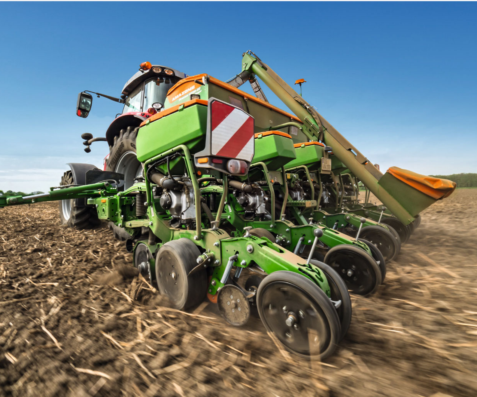
Precea 4500-2CC precision air seeder in work
