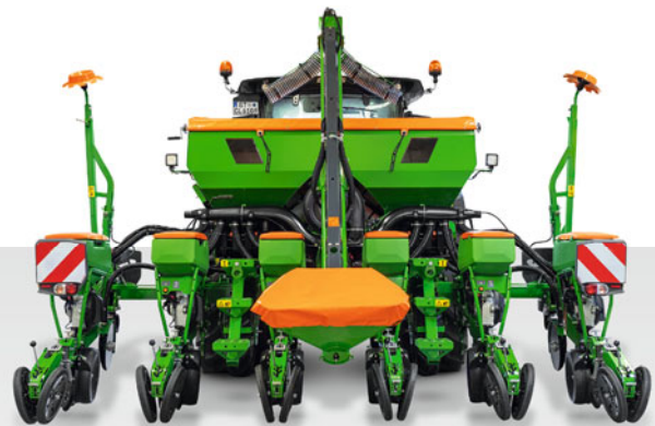
The Precea 4500-2CC with its variable telescopic frame at full working width
