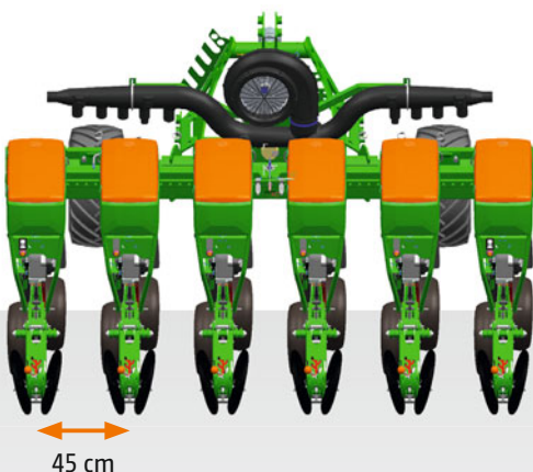
The variable telescopic frame on the Precea 4500-2 and 4500-2CC
