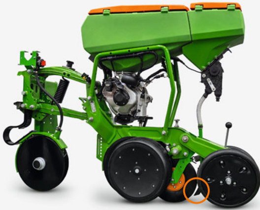
Micro micro-granular applicator with distribution point in the row
