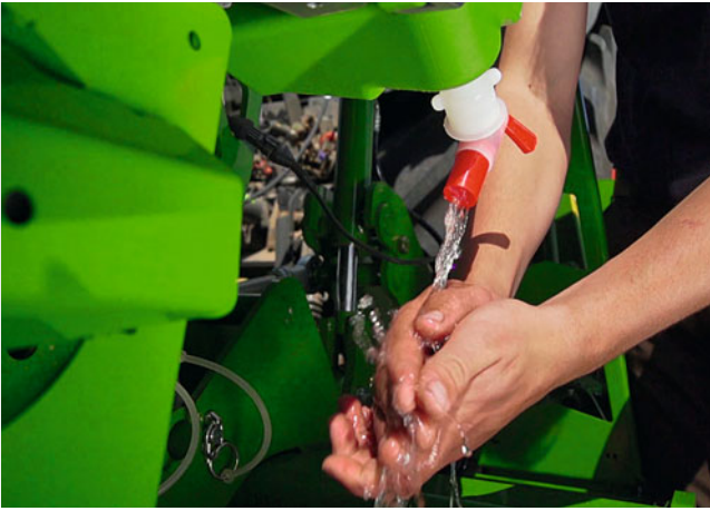
✓ Hand wash tank
