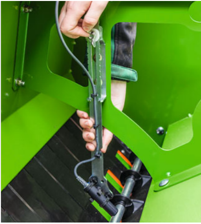
The simplest of conversion from fine to normal seeds via the shutter slide
