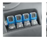
Functions such as open/close maize header and pick-up support wheels, header tilt, lift/lower discharge chute are conveniently controlled using the toggle switches.
