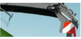
Powerful LED work lights on discharge chute available as an option.
