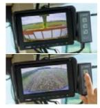
When driving forward, you can see the fill level of the accompanying vehicle through the camera on the discharge chute. When reversing, the image is automatically switched to the reversing camera.
