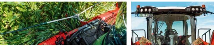
The maize header is available with eight, ten or twelve rows. For on-road driving, the header folds up hydraulically, so it can be brought into transport position quickly.
